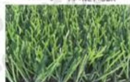
SHA-23420 Type: PRO-2-5016 Pile height: 50 mm Stitch Rate: 16 /10cm Gauge: 5/8 inch Density: 10080 stitches/m 2 Dtex: 8800 Backing: PP+NET+SBR
